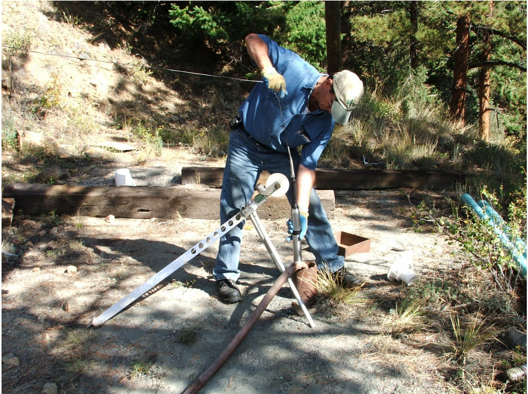
Lowering seismic source into Borehole U1. Note water hose used to fill borehole.
