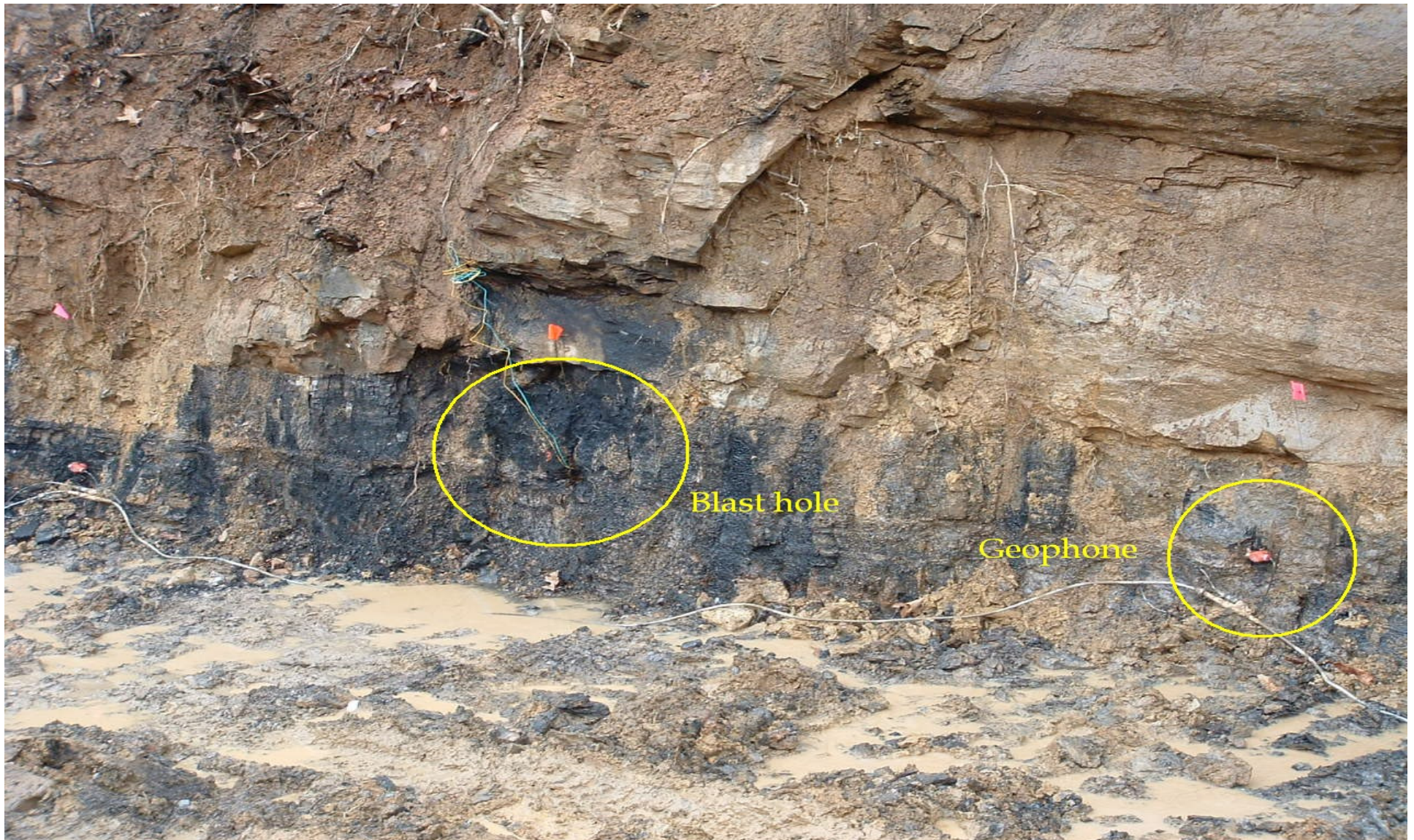
View of charged blast hole and geophones placed into the face of the coal outcrop.
