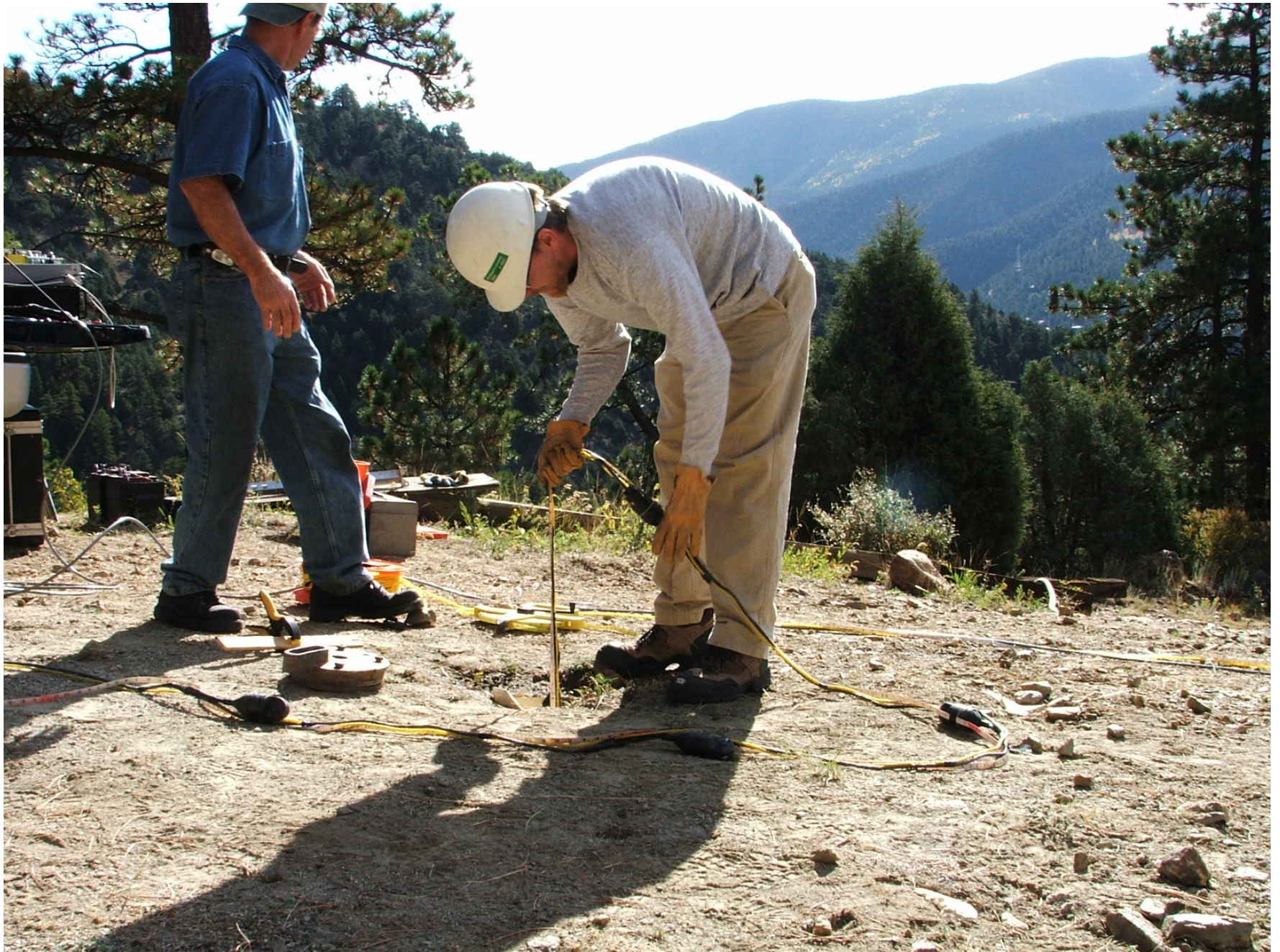
Lowering hydrophones into Borehole U5
