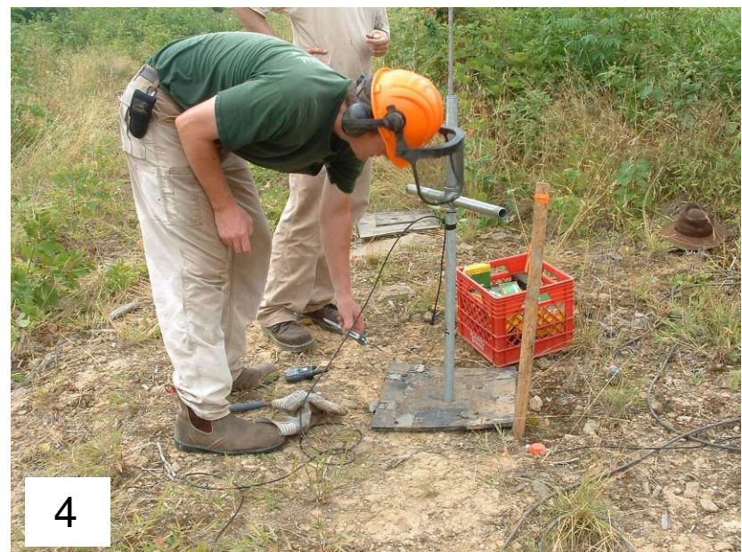
(1) Assistant puts shotgun shell in fitting and hands to firer; (2) firer screws fitting and shell onto end of pipe; (3) “seisgun” is lowered into hole; and (4) rod is placed in pipe. The “seisgun” is ready to be fired by striking the end of the rod with a hammer.
