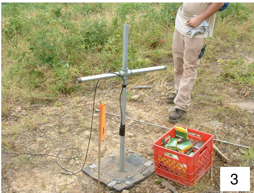
(1) Assistant puts shotgun shell in fitting and hands to firer; (2) firer screws fitting and shell onto end of pipe; (3) “seisgun” is lowered into hole; and (4) rod is placed in pipe. The “seisgun” is ready to be fired by striking the end of the rod with a hammer.
