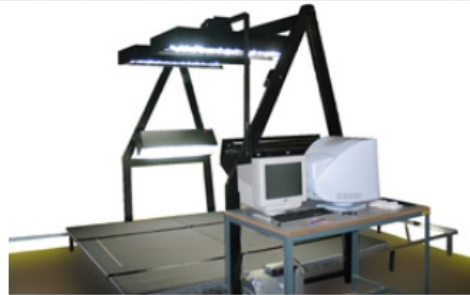
Icam's large format document handling camera
